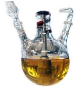
Sensorsystem (im Ölbad) zur Ölzustandsüberwachung Sensor System (in oil bath) for Oil-Condition-Monitoring
